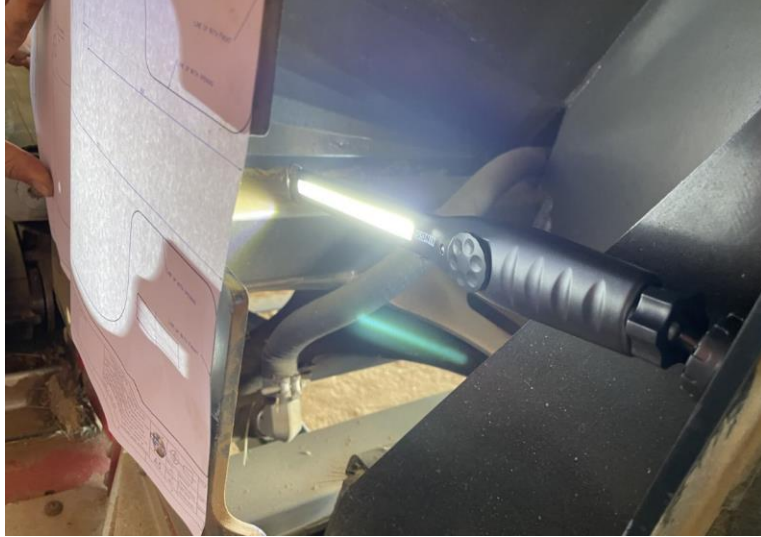
Figure 6: Drill Template position in front.
