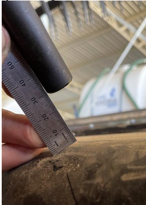
Figure 9: Measure the clearness between the finger and center draper.
