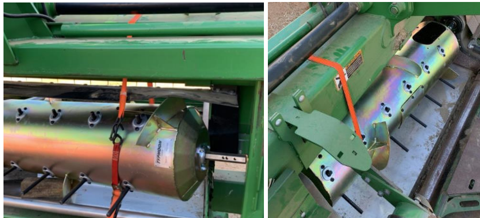
Figure 1: Securing the feed drum with a ratchet strap.
