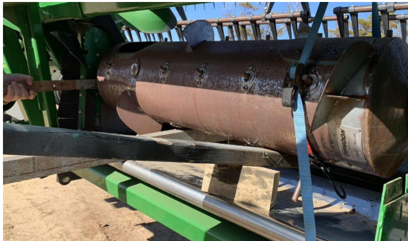
Figure 8: Using wooden beams to lever and maneuver the drum shell.
