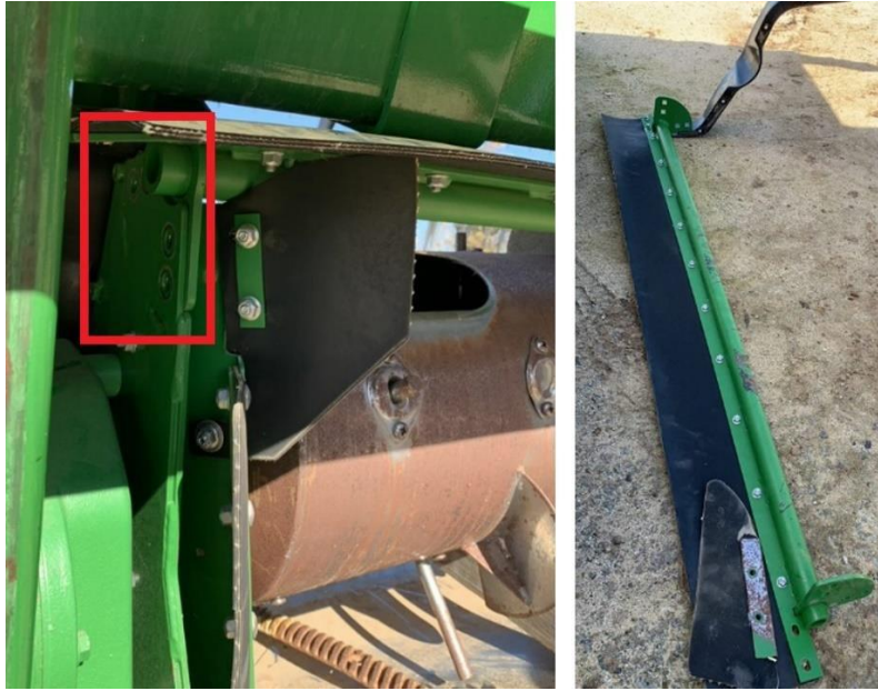
Figure 5: Removal of bolts securing top cover on drive side (left). Top cover removed (right).
