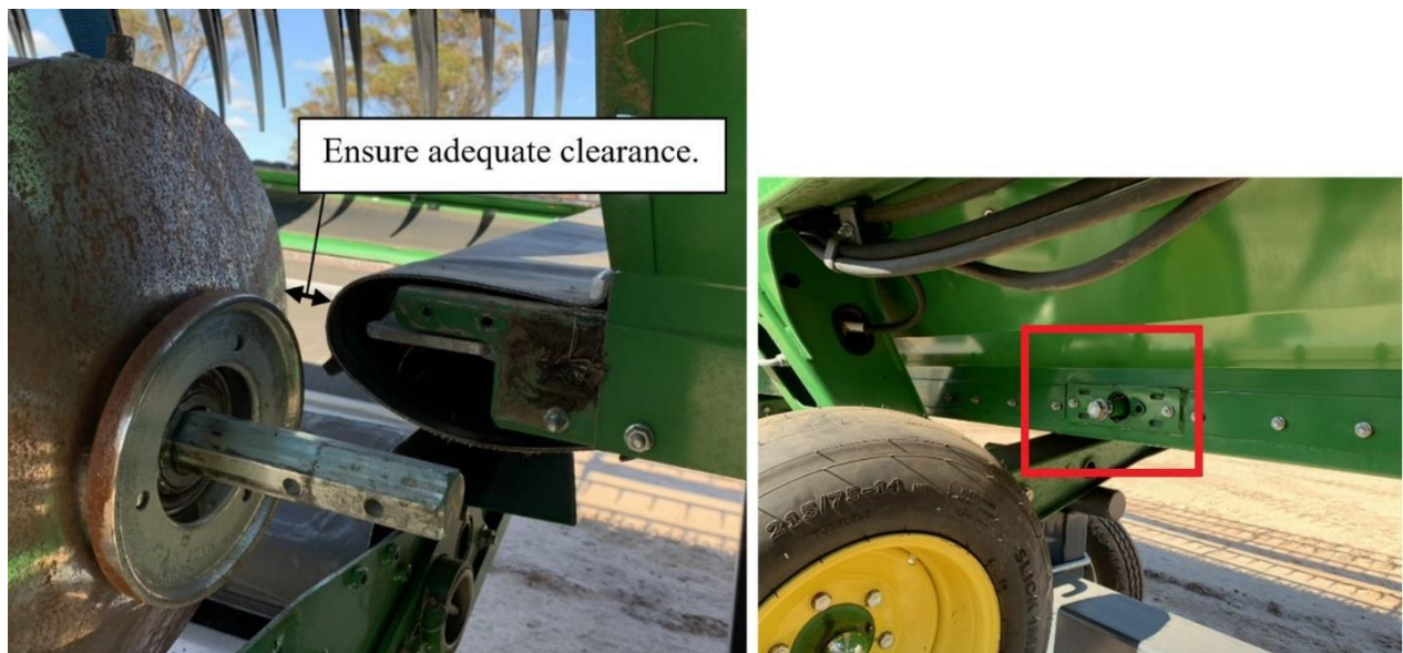
Figure 6: Clearance between the drum and Draper belt (left). Bolt (shown in red) used to move the Draper belt (right).
